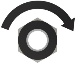
TIGHTEN UNTIL SPRING LOCK WASHERS ARE FLAT
