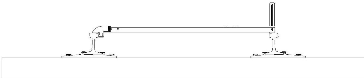
Take note to the position of the bubble. Is it to the right or left of center? How far from center or one of the indicator lines is it?
