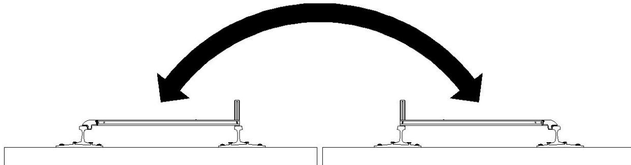
Using a Phillips screwdriver adjust the vial so the bubble is located in the same position noted before turning it end-to-end. Note the new location of the bubble.
