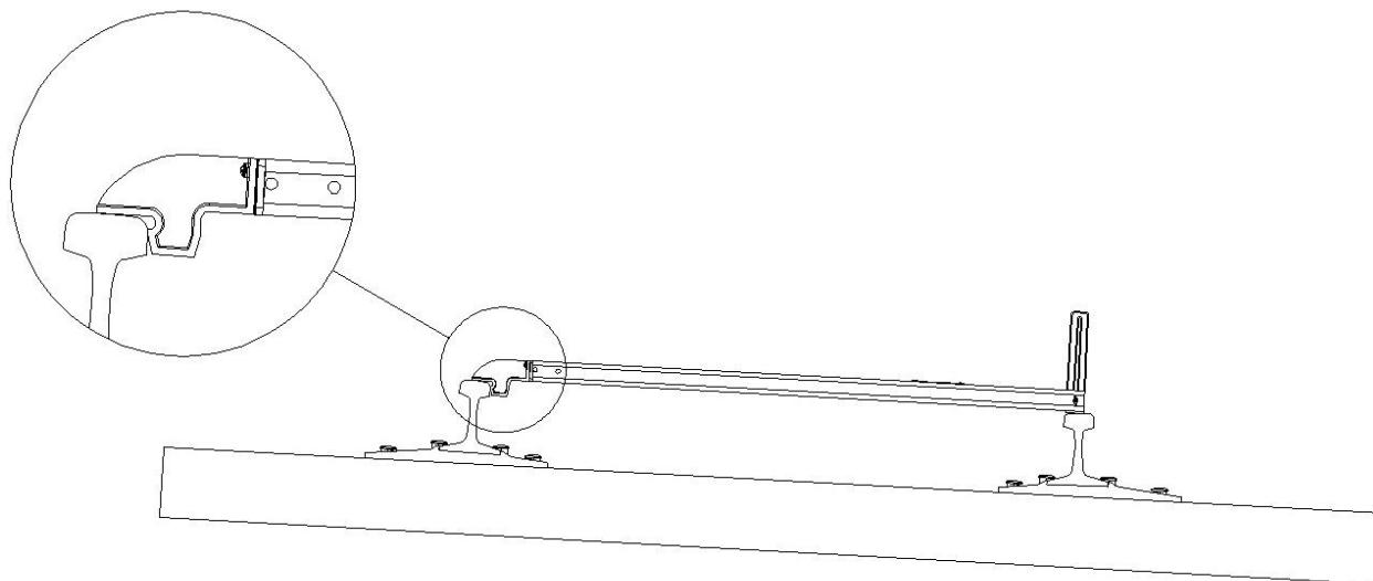
With the wing nut loose lift the super-elevation end of the level (with the super-elevation scale on the rail) until the bubble reads plumb. Tighten the wing nut.
