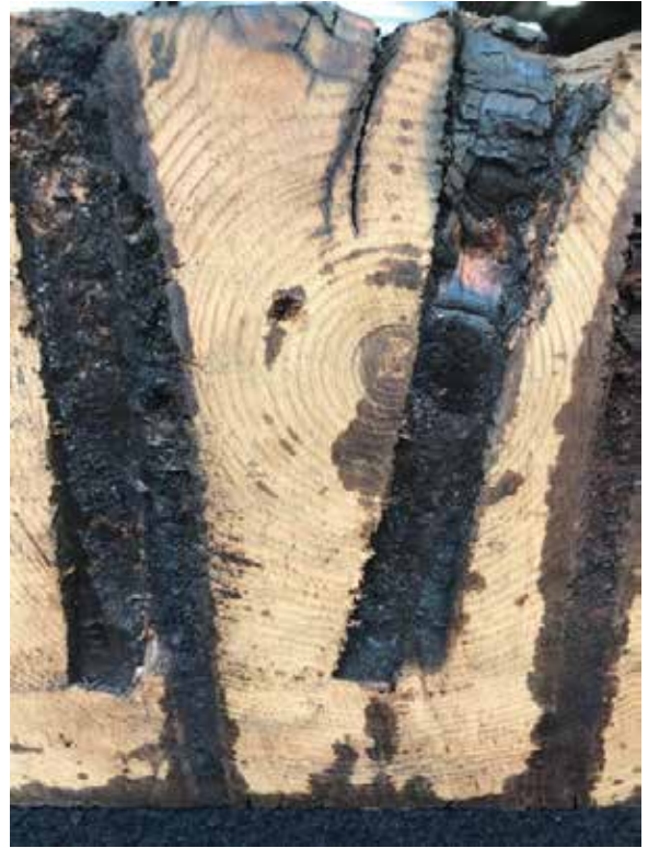
Spike extracted - note visible melting to tie
