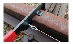
**3.** Attach the spool to the other paddle's hook and walk the paddle down the rail until the reel stops.
