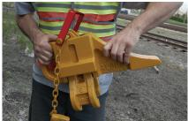
**2.** Place the block over the rail head, allowing the clamps to fall around the head.
