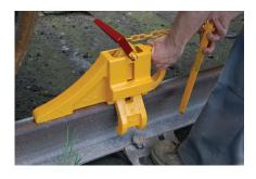
**3.** Pull up on the clamp handle to allow the clamps to lightly cusp the rail head. Loosely install the wedge to hold the clamps in position.
