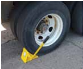
8 30" Handle makes installation easy.
