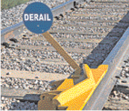
Derail with Blue Sign
