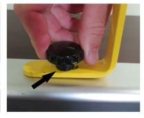
With the handle fully assembled, position it on top of your track gauge. Align the oval shaped hole on one end of the handle over the rivet nut and fasten it securely to the track gauge using a thumb screw. Repeat the same process on the other end of the handle.
