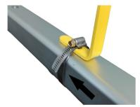
Using a 5/16" socket wrench, completely open the hose clamp. Position the hose clamp over the handle and track gauge, tighten the clamp until the handle is secure. Repeat the same process on the other end of the handle. **The hose clamps allow the universal handle to be attached to almost any track gauge or elevation level.**
