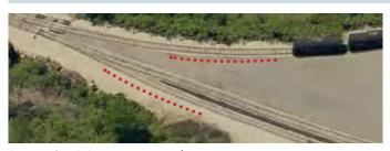
RAIL KICKER Braces are good insurance against gaugewidening for curved track entering or leaving a switch, where wheel side pressure can be at its greatest.
