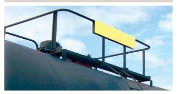
Fits over gap in railing on top of tank car. Formed aluminum panel, 48" wide drops over railing. Handle provided on top of panel.
