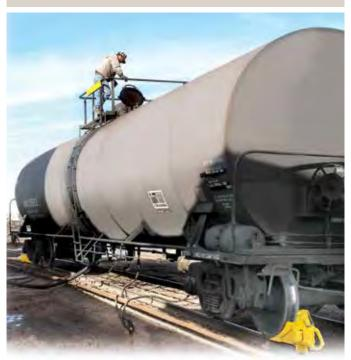
A "super" chock, cast in ductile iron. Use at each end of car for secure blocking. Can be used on flush rail provided flangeway is created on field side of rail.
