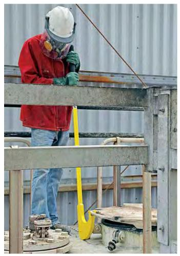
**Much better than a crowbar!** Designed to engage the grab-handle of tank car manway covers. Five-foot handle and a rocking foot provide the leverage to overcome suction caused by the difference in atmospheric pressure outside the tank car and inside.
