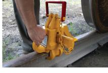
**5.** Drive the wedge home using a suitable size hand sledge hammer.
