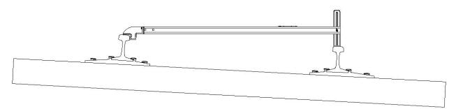
Read the measurement from the top of the main body tube against the scale. This measurement directly indicates super-elevation.
