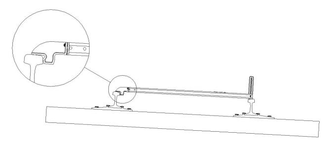
With the wing nut loose lift the super-elevation end of the level (with the super-elevation scale on the rail) until the bubble reads plumb. Tighten the wing nut.
