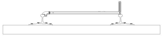
Take note to the position of the bubble. Is it to the right or left of center? How far from center or one of the indicator lines is it?
