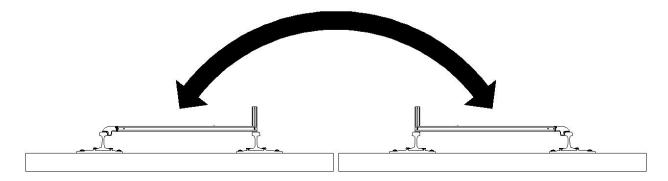
Using a Phillips screwdriver adjust the vial so the bubble is located in the same position noted before turning it end-to-end. Note the new location of the bubble.
