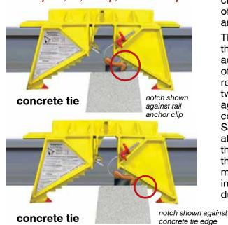
2. For wood or concrete tie track, ties must be at least 19 in. apart on centers. Dig away enough ballast on each side of the tie so derail can lie flat on the rail and a tie brace notch of either step bar can engage the edge of the tie plate or a tie clip (wood tie) or edge of concrete tie or the rail anchor clip.
