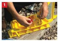
BEFORE INSTALLATION: Remove locking pin, release locking arm, and replace pin.
