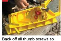
Back off all thumb screws so that 1/2" or less of threading shows inside housing.
