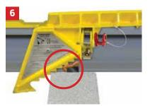
FOR CONCRETE TIES: Seat tie brace notch against the edge of full length concrete tie or against the rail anchor clip.
