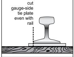
create an insecure foundation for the derail.
