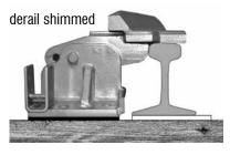
note that "height of rail" includes tie ADJUSTMENT plate thickness HEIGHT DERAIL NOTCH SHIM OF RAIL SIZE TIE DERAIL 6 5/8" ...... 7 ...... 3/8" 6 3/4" ...... 7 ..... 1/4" 6 7/8" ...... 7 ..... 1/8" 7 1/4" ...... 7 ...... 1/4" 7 1/2" ...... 7 ...... 1/2" 7 5/8" ...... 8 ...... 3/8" 7 3/4" ...... 8 ..... 1/4" 7 7/8" ...... 8...... 1/8" 8" ...... 8......- ........-8 1/4" ...... 8 ...... 1/4"
