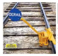
ALWAYS Lift up sign when you place derail block on rail. Lower sign when you throw derail block off rail.
