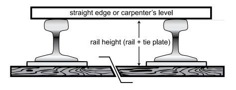
NOTE: make sure there is no gap between rail, tie plate, and tie. Any such "daylight" must be removed by lifting the tie and re-tamping
