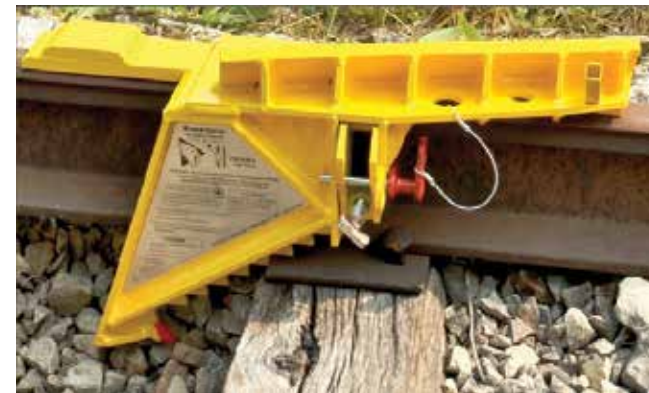
One-way derail shown contacting tie plate of wood tie
