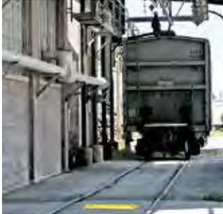
Designate where railcars are to be spotted on spur track. Mark locations of dumping conveyors.
