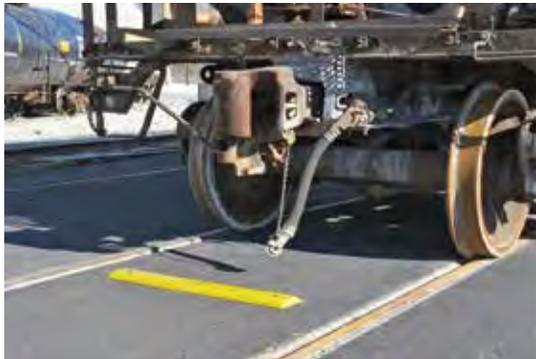
Low-profile bright yellow urethane marker to indicate parking limits on tracks encased in concrete or asphalt.
