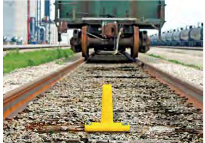
The Aldon® Track Clearance Marker tells switching crews how far they can shove a car without "fouling" converging tracks.
