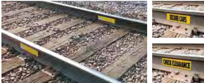
For temporary or permanent marking on both sides of rail web to show limit of car shoving on a siding. Can also be used to mark loading/unloading sites. Fits rails 90-142 lbs./yd.
