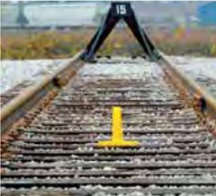
Protect bumping posts and car stops by marking one car length ahead to signal: "Slow down! Get ready to stop!"
