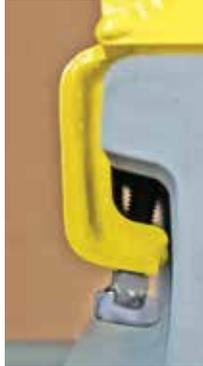
5. Tighten locking arm screw and then tighten all three screws on field side. **All four screws must be tight. Derail must be level and straight.**
