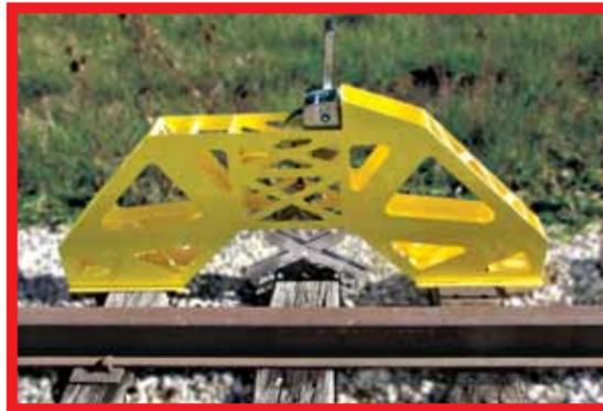
A more efficient way to secure a replacement tie for re-spiking. Takes the place of old-fashioned nipping bars. Grab tongs, operated by a hand crank, pull tie up against rail base so rail can be spiked firmly.
