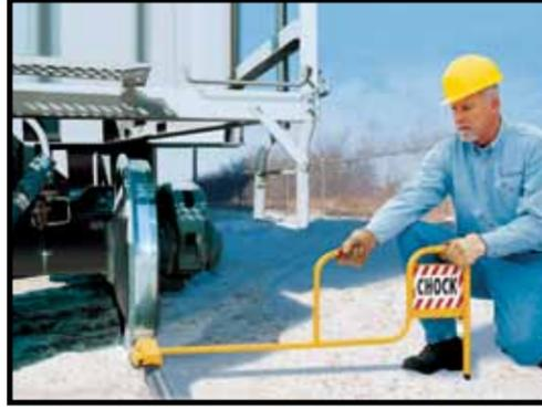
Keep your head and hands away from the rail car when placing wheel chocks. Handle length 44".
