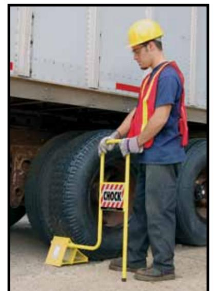
**Walk-In Wheel Block.** Keep hands and body clear of trailer when placing aluminum wheel block under tire. Chock sign is more visible to driver in truck cab.
