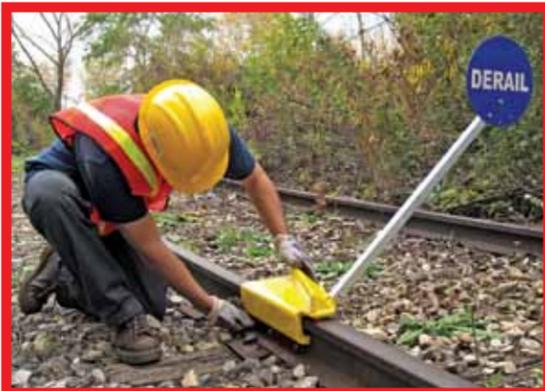
**Sabertooth™ Portable Derail** weighs only 35 lbs. No wrenches needed to install. Safety hook bites into tie to keep derail from sliding.
