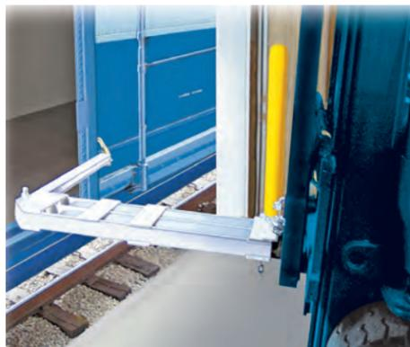
erator makes a series of arc-like movements which first tug, then push the door open or closed. The Easy-Slide design meets the the OSHA conditions for acceptable use of a fork truck to open and close box car doors.
