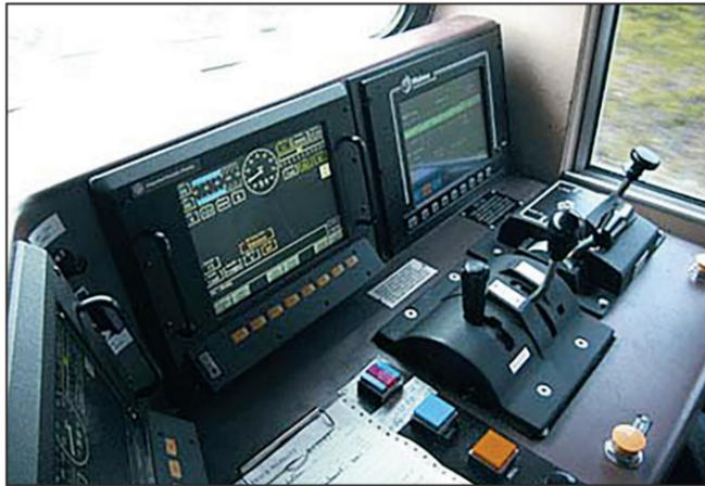
**Inside the locomotive cab, PTC computers monitor and advise the locomotive engineer on every aspect of train operation.**
